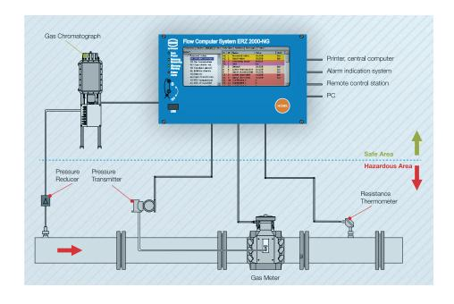
The ERZ 2000-NG base module performs neutral measurements of all inputs similar to a multimeter, but no calculations or assignments to physical units are made.
